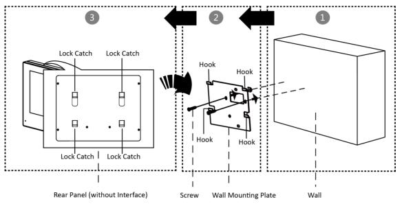
Figure 5-3 Wall Mounting without Junction Box
