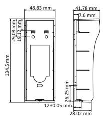
Figure 5-4 Wall Mounting Shield
