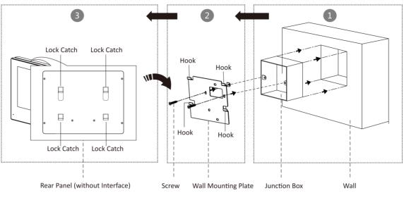
Figure 5-2 Wall Mounting with Junction Box
