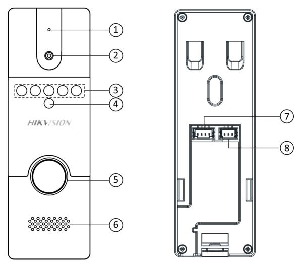
Figure 3-2 Appearance of Doorphone
