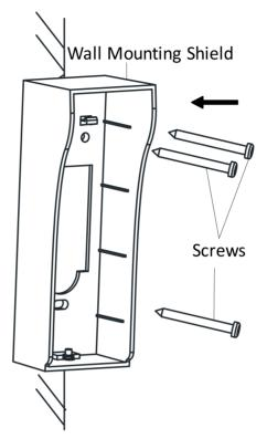
Figure 5-5 Fix Shield to Wall
