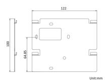
Figure 5-1 Wall Mounting Plate
