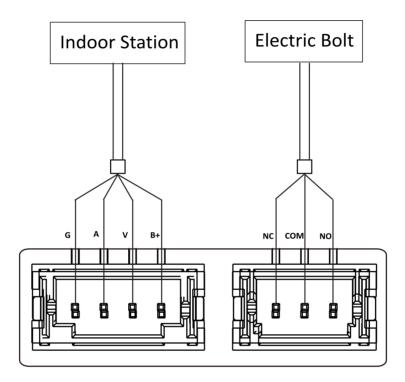
Figure 4-2 Terminal of Doorphone
