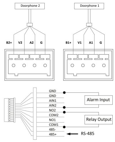
Figure 4-1 Terminal of Indoor Station
